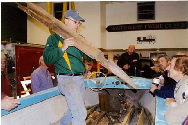
Kenny Heaton Shows Rotted Support Member and Replacement Piece Ready for Sealing and Installation
