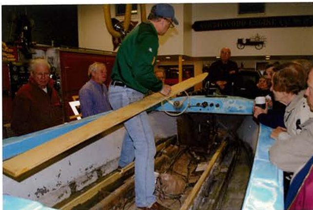
Kenny Heaton Shows Rotted Support Member and Replacement Piece Ready for Sealing and Installation
